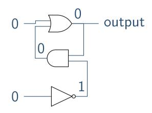
Note that this is stable. But two different stable outputs are possible with input (0,0).
