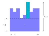
t is the length of the job starting at  $\ell$ and ending at the makespan T is the total length of all jobs Define  $V = \ell \cdot m$ Now conclude: OPT  $\geq T/m$  and OPT  $\geq t$  $T \geq V + t$ , due to Ls's choice for t
