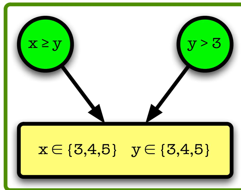
constraint store with connected propagators
