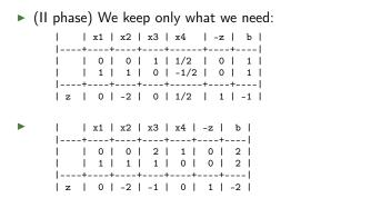
Optimal solution:  $x_1 = 2, x_2 = 0, x_3 = 0, x_4 = 2, z = 2$ .
