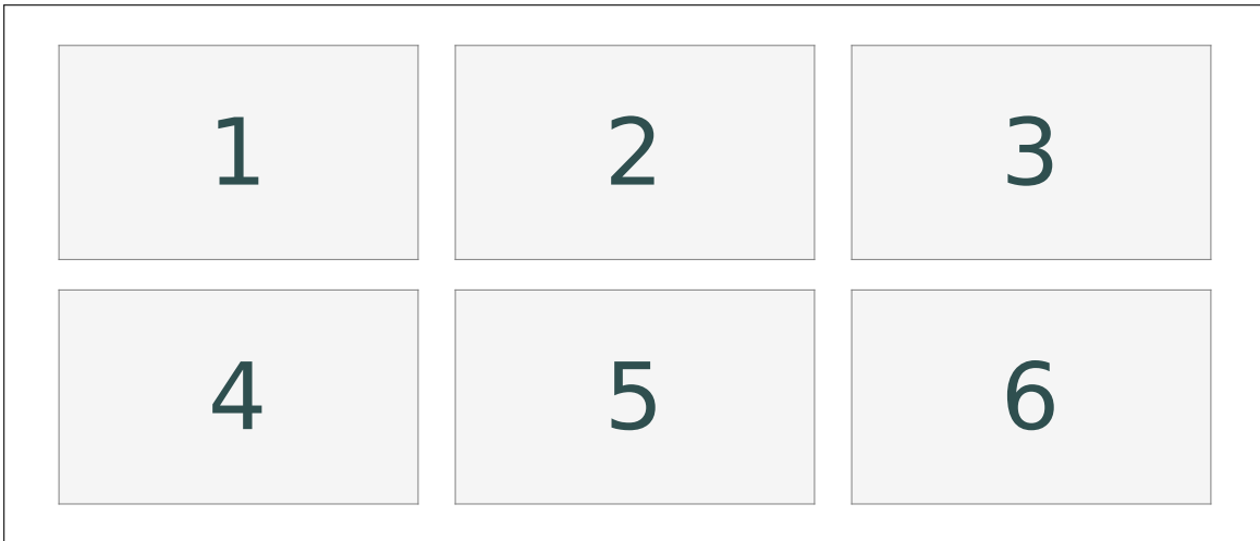
Figure 5.3: The layout of subplots with plt.subplot(2,3,i) (2 rows, 3 columns), where i is the index pictured above. The outer border is the figure that the axes belong to.
