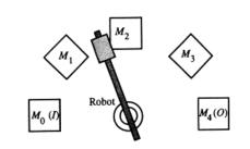
Search for periodic pattern of moves (cycle) *one-unit cycle:* the robot load (or unload) each machine exactly once *k-unit cycle:* each activity is carried out exactly k times
