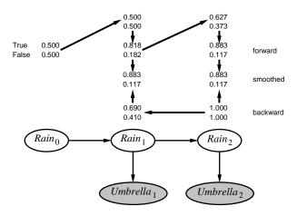
Forward–backward algorithm: cache forward messages along the way Time linear in t (polytree inference), space  $O(t|\mathbf{f}|)$
