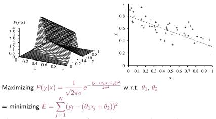
That is, minimizing the sum of squared errors gives the ML solution for a linear fit assuming Gaussian noise of fixed variance
