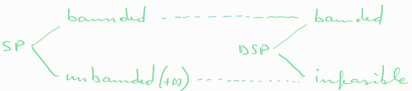
If SP bounded and DSP bounded, then the solution of DSP will be in one of the extreme points by the fundamental th. of lin. programming. Hence:
