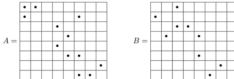
Given are the two sparse matrices  $A$  and  $B$ . Consider the problem of sparse matrix-matrix multiplication. A dot corresponds to a non-zero entry. The computation is decomposed into 8 tasks. Let task  $i$  be the owner of row  $A[i, *]$  and of row  $B[i, *]$ . Task  $i$  has to compute row  $i$  of the result  $C = A \cdot B$ .
