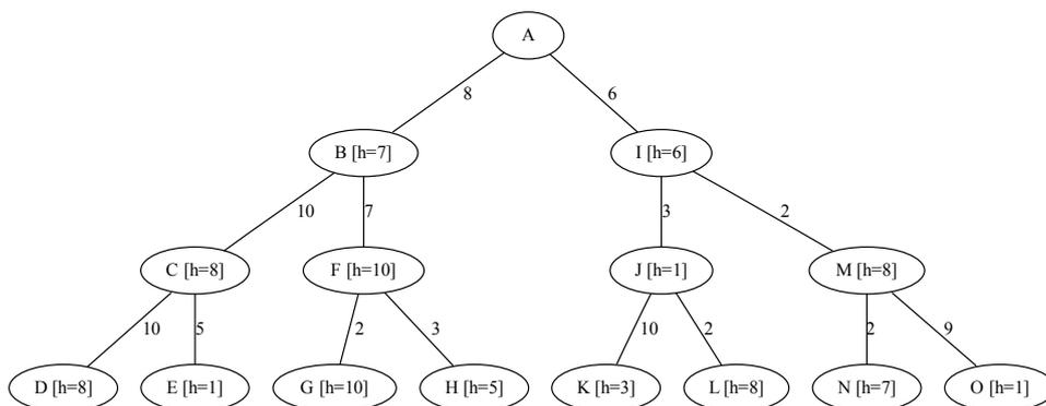
Figure 1: Values on the edges represent step costs and values on the nodes the heuristically computed value of completing the solution from that node.
