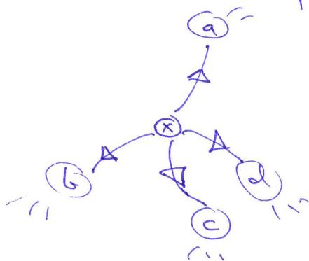
$$\left[ \begin{array}{l} \vdots \\ (x, a) \\ (x, b) \\ (x, c) \\ (x, d) \\ \vdots \end{array} \right]$$
