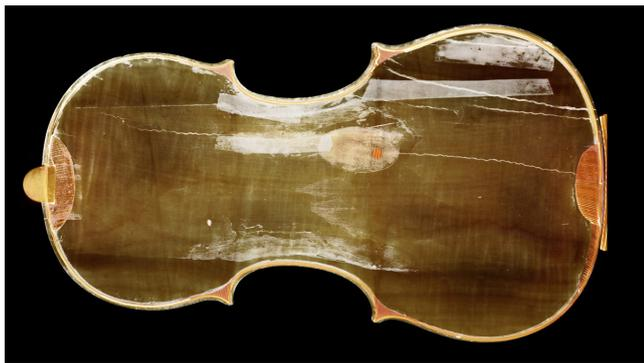
**Figure 20:** A colored three-dimensional visualization of a violin scanned by computed tomography. The color transfer function highlights glued areas (bottom) [Hop18].
